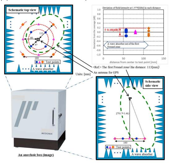
The uniformity is excellent because our anechoic boxes have been well-designed and properly manufactured in rich experience.
