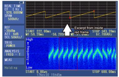
By displaying the frequency vs. time, it is possible to observe the frequency bandwidth and transmission time of the chirp signal.
