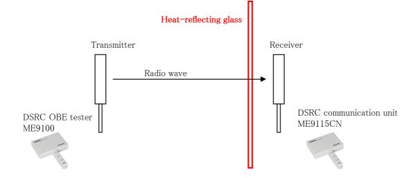
OBy comparing the data with that of the reference glass used without problems ETC/DSRC communication, check whether the radio wave transmitted.
