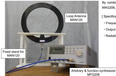
By combining the loop antenna MAN120 and the function synthesizer MAG206, the following frequency and output level can be handled.
