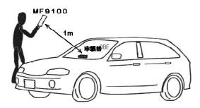
Moreover, ME9100 is opposed in parallel to OBE and the test is performed 1m away(range from 0.8 to 1.2m), as shown in figure. When the communication test is performed in this state, the radio wave strength of OBE can be checked simultaneously. If the test result is "Pass", the radio wave strength of OBE is normal. If "Pass" is displayed at distance below 0.8 m, cable wiring or OBE itself should be rechecked because radio wave level is low.
