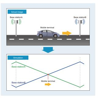
It simulates the attenuation process of radio wave in which the communication of mobile terminal transfers from base station A to base station B.
