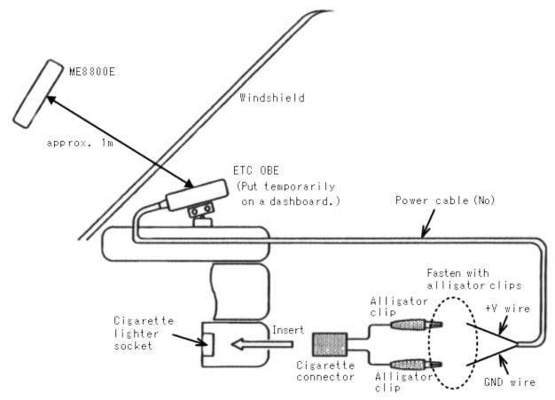
Place the ETC OBE to be installed on the dashboard. Fasten the +V wire and GND wire of the power cable coming out of the ETC OBE with alligator clips, and insert the cigarette connector to the cigarette lighter socket. The ACC wire is added to ETC OBE of some kind. In such a case, connect the ACC wire and +V wire together, and fasten them together with an alligator clip.
