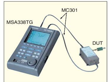
Fig.1 Connection for measurement
