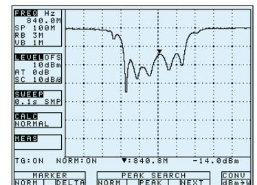
Fig.4 Waveform of return loss
