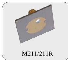
This is a right circular polarization antenna used in the ETC/DSRC. There are two types of the Reference antenna (M211R) and the Transmission Receiving antenna (M211). The antenna gain and VSWR data are attached only to the Reference antenna.
