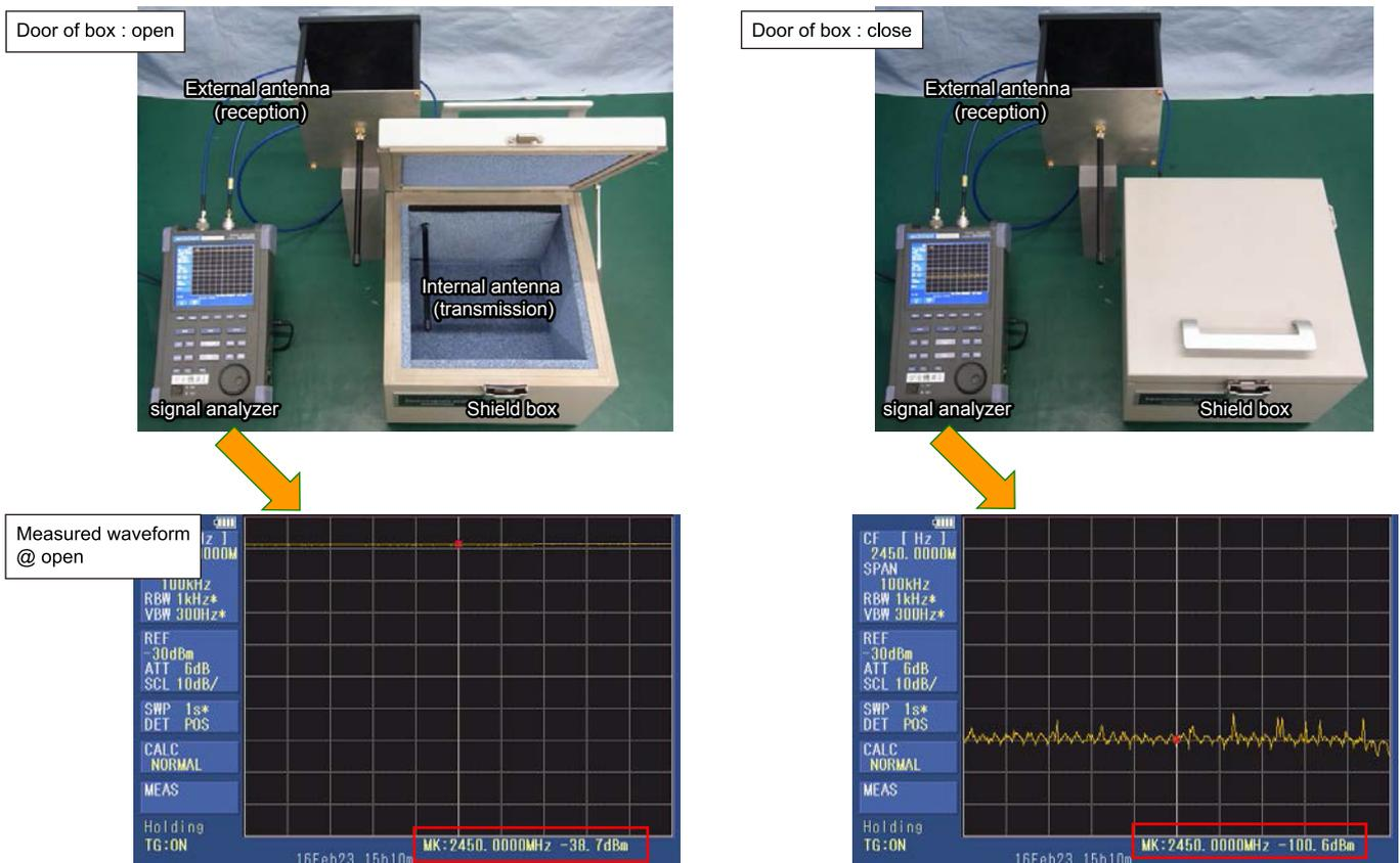
In the connection example, when opening the door: -38.7dBm @ 2450 MHz, but when the door is closed: -100.6dBm @ 2450MHz. However, the measured value of "-100.6dBm" which is the reference value is important. It is judged that the shielding performance deteriorates if the electric field strength level goes upper than this reference value.
