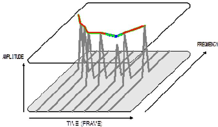
The spectrogram displays the time response of frequency and power by X-Y axis and by X-Z axis respectively. Z axis is expressed by colors.
