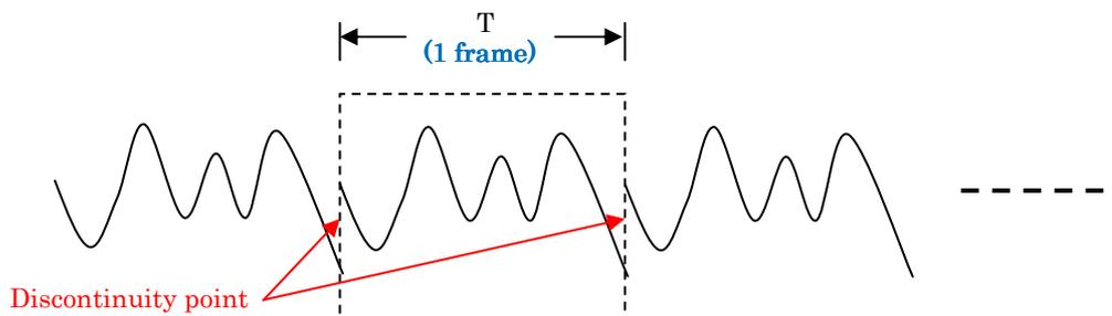
The calculation of Fourier transform is performed as the signal captured during T seconds is repeated.
