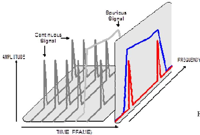
OverWrite is a function in which the spectrum waveform of each frame is piled up and then displayed. The spectrum waveform is continuously accumulated at the rate of **720 frames/sec**. The occurrence frequency is expressed by colors.
