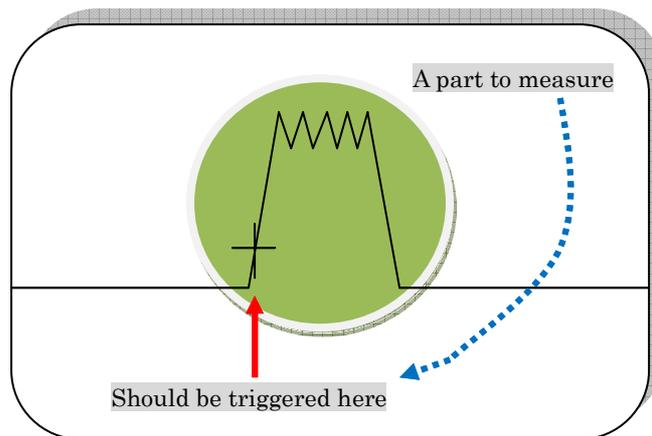
The capturing range of a waveform is determined by Trigger, Pre-trigger and Span.
