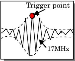
When the level of IF signal (modulated with 17MHz) crosses the trigger preset value, the trigger signal is generated. The slope "rising" or "falling" is not available.
