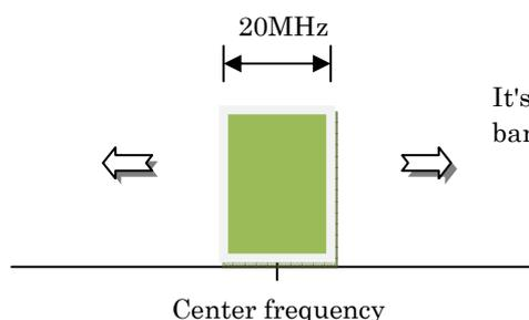
It's possible to move to any frequency band if the center frequency is set.
