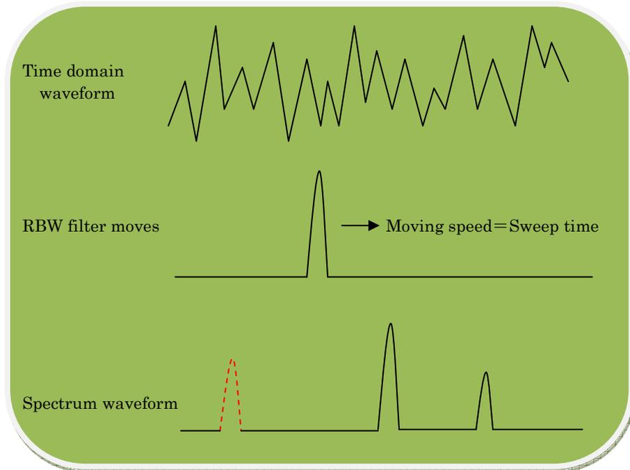
One RBW filter **moves** in the sweep range specified and then spectrum is displayed.
