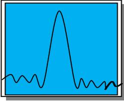
When the instantaneous value of whole power in the screen crosses the trigger preset value, the trigger signal is generated. The slope of "rising" or "falling" can be also set.
