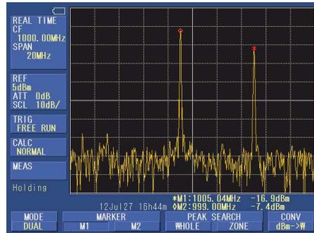
The bin expresses frequency resolution and every span consists from 602 bins (a part of 1024 bins by FFT operation).
