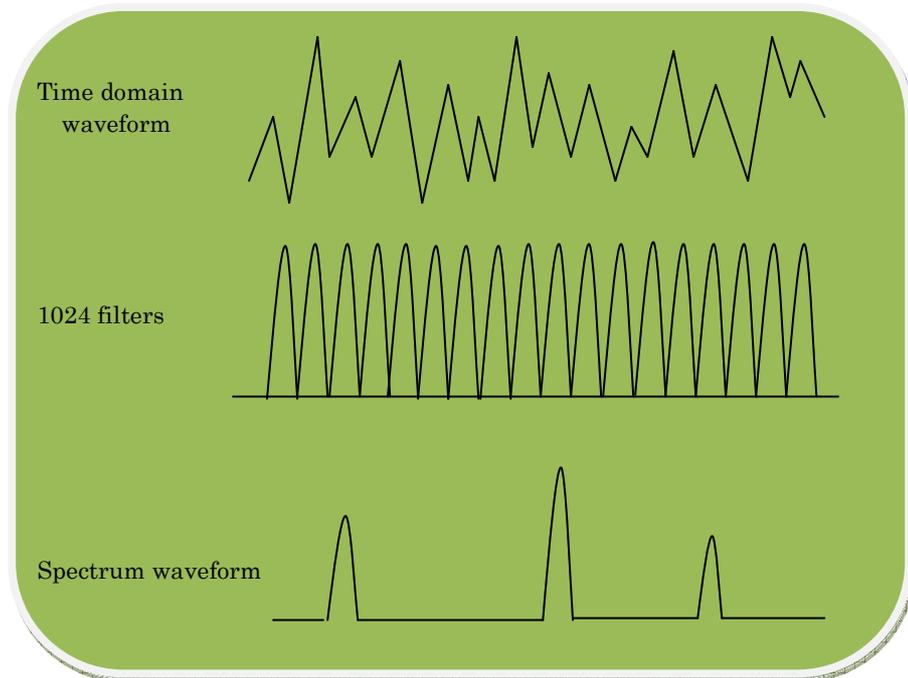
Many filters (1024 filters in MSA500) are arranged in parallel.
